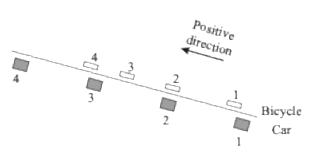
In the car's frame, the bicycle has a greater displacement for each consecutive time interval. Thus, the bicycle is speeding up as it moves down along the hill relative to the car.
