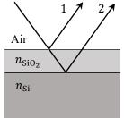
6. [5 pts] The figure at right shows part of the solar cell with the silicon oxide coating. A ray is incident normally (shown incident at angle for illustration).
