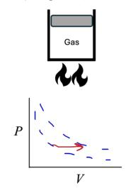
16. [5 pts] The *PV*-diagram shows two different processes, A and B, connecting two states of a sample of ideal gas. The initial and final temperatures of the states are the same (i.e.,  $T_i = T_f$ ).
