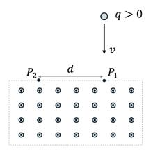
The trajectory of the particle will be a half circle with diameter 2r = d. Thus, the answer is double the radius of a particle's path in a magnetic field: d = 2r = 2mv/(qB).
