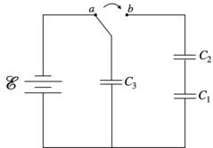
15. [5 pts] What is the effective capacitance of the circuit after flipping the switch to position **b**? Show your work.
