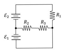
We apply the Kirchhoff's loop law, going through the larger loop to calculate the voltage across  $R_1$ as:  $\mathcal{E}_1 - \Delta V_{R_1} - \mathcal{E}_2 = 0 \Rightarrow \Delta V_{R_1} = \mathcal{E}_1 - \mathcal{E}_2 = 10 V$ .
