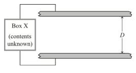
18. [5 pts] When the top plate is moved closer to the bottom plate, does the absolute value of the charge density on the top plate *increase*, *decrease*, or *remain the same*? Explain.
